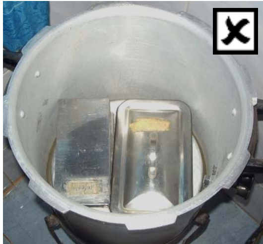
Figure 26 Example 1 of incorrect packing of steam sterilizer
