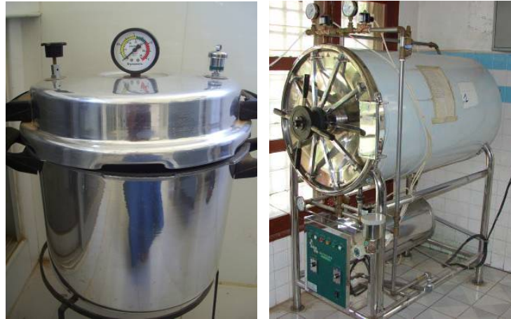
Figure 24 Pressure cooker sterilizer and autoclave
