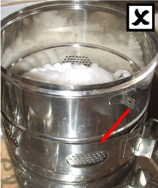
Figure 28 Incorrect storage and packing of gauze drum.
