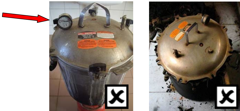
Figure 29 Examples of poorly maintained sterilizers
