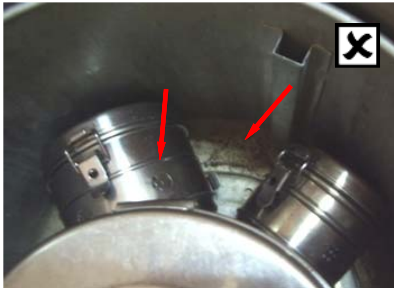
Figure 27 Example 2 of incorrect packing of steam sterilizer. Please also note 1) ventilation holes are closed and 2) the dirty pressure cooker
