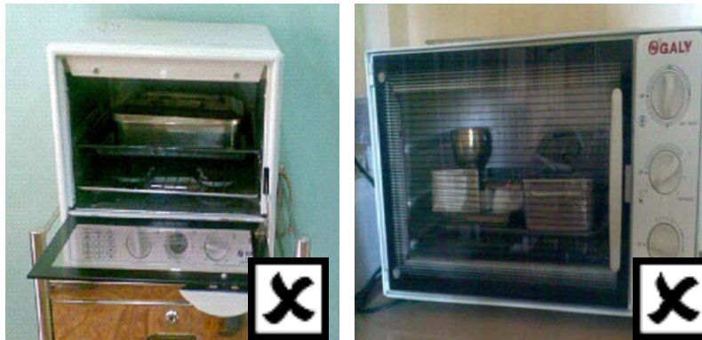
Figure 30 Examples of inappropriate ovens for dry-heat sterilization Ovens are domestic ovens and should not be used for medical purposes
