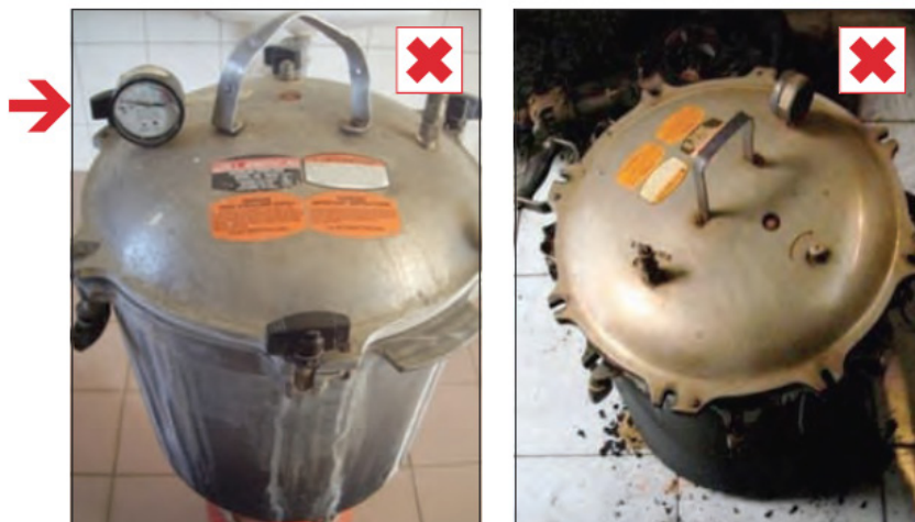
| Figure 85 Examples of poorly maintained sterilizers
