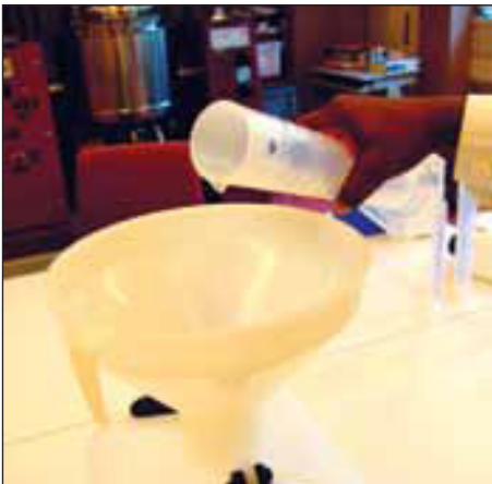
2. Hydrogen peroxide is added using the measuring cylinder.
