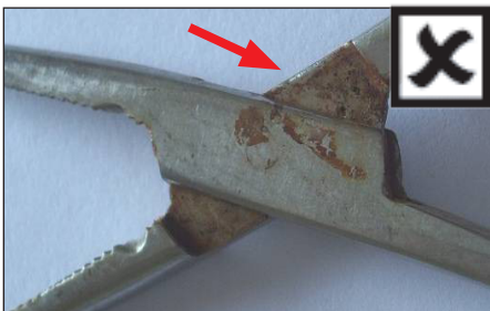
| Figure 32 Insufficient Cleaning and damaged equipment
