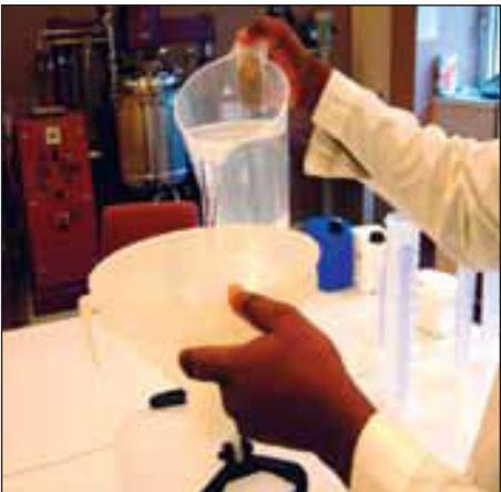
1. The alcohol for the formula to be used is poured into the large bottle or tank up to the graduated mark.
